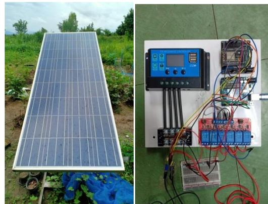
Figure 2. Prototype of watering cassava crop systems through smart Phone
